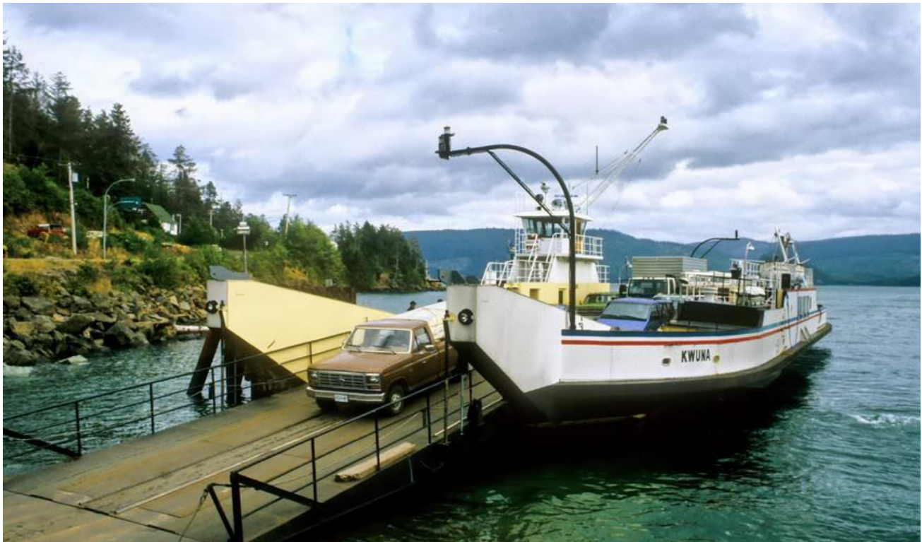
Example of a K class vessel using a 'landing craft' ramp configuration
